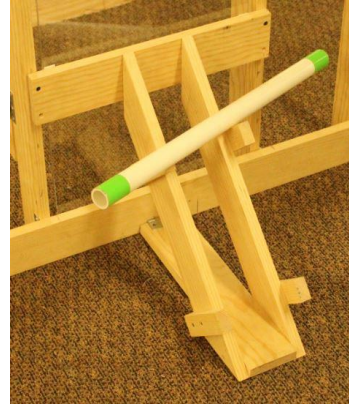
Correct 7: Core Sample is completely Supported by both sides of the upper shelf. (Incidental contact with the slanted sides is allowed)
