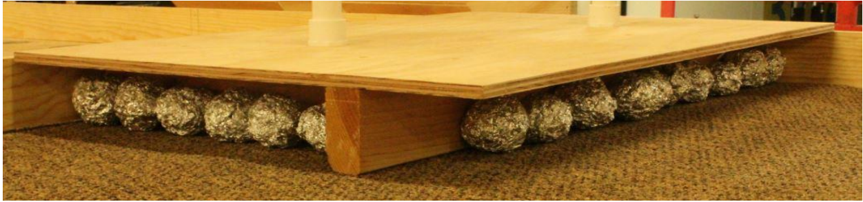
Figure 1 – Correct, all pieces are in contact with a 2x4, and underneath platform.
