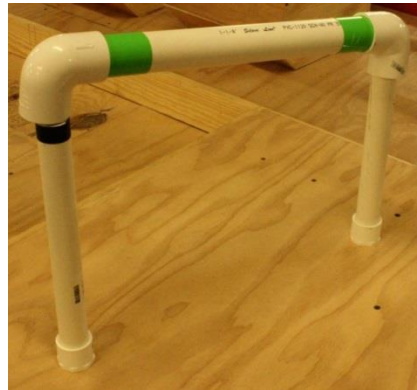
Incorrect 10: RP only covering one tape line.
