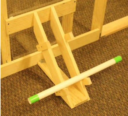
Correct 6: Core Sample is completely Supported by both sides of the lower shelf. (Incidental contact with the slanted sides is allowed)
